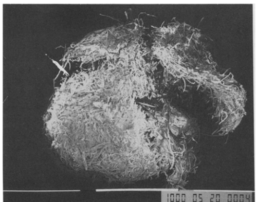
Fig. 3. Special cellulose bead, 1.1 mm diameter, prised apart. Scale bar represents 1 mm.
